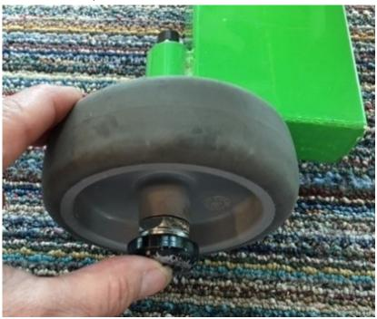
• Replacing the wheels – When pushing the wheels back onto the frame, be sure that the small pin goes all the way through and engages so that the wheel is locked in place.
